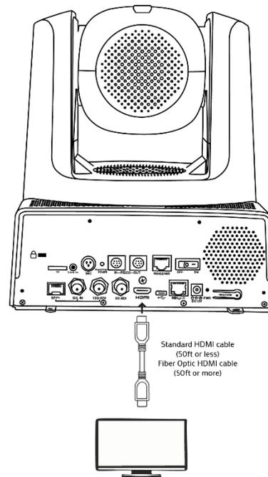
**1** Connect HDMI cable to the output of the PTZ camera, and into your HDMI ingest. Video should appear after a slight delay.
