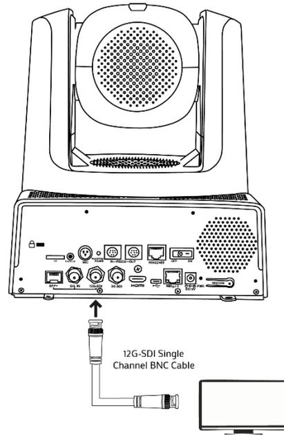
**1** Connect the BNC SDI cable to the 12G-SDI output slot. Connect the other end of said BNC SDI cable to your SDI ingest.
