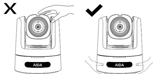
⚠ Please install the camera on a smooth, fixed surface free from vibrations. Avoid placing on slanted or leaning platforms. Optional ceiling mount (CM-PTZ12G-B/W) and optional wall mount (WM-PTZ12G-B/W) are recommended and sold separately.
