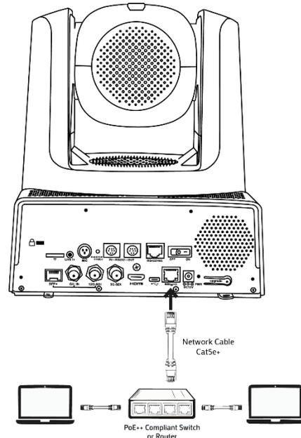
**1** Connect a ethernet cable (cat5e or better recommended) cable to the back of the “NDI® HX” port. Connect said cable to your local network switch.
