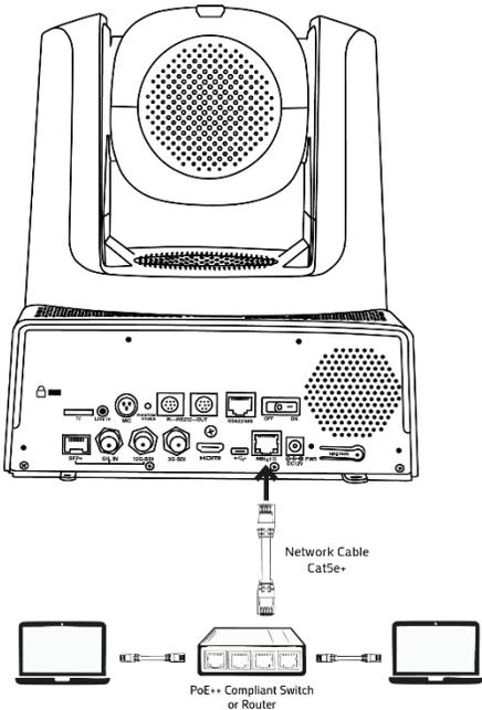
**1** Use a Cat5e or better patch cable to connect to a PoE++ compliant switch or router.
