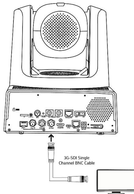
**1** Connect a 3G-SDI BNC cable to the 3G-SDI port on the back of the PTZ. Connect the other end of said BNC SDI cable to your SDI ingest.
