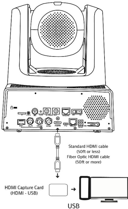
**1** Connect HDMI cable to the output of the PTZ camera, and into your HDMI capture card.
