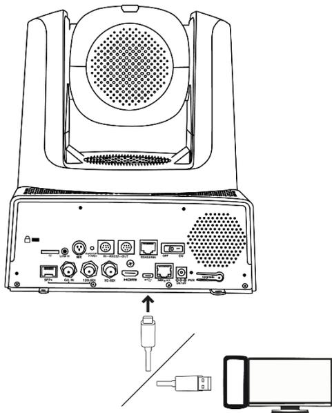
**1** Use the supplied USB-C type cable, or identical USB-C type cable to connect directly to a PC. The PC should show up as a webcam.
