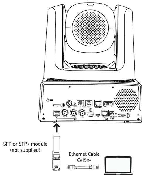
**1** Place the SFP or SFP+ module (not supplied) into the SFP+ cage on the back of the PTZ. Securely place it until an audible \*click\* is heard.
